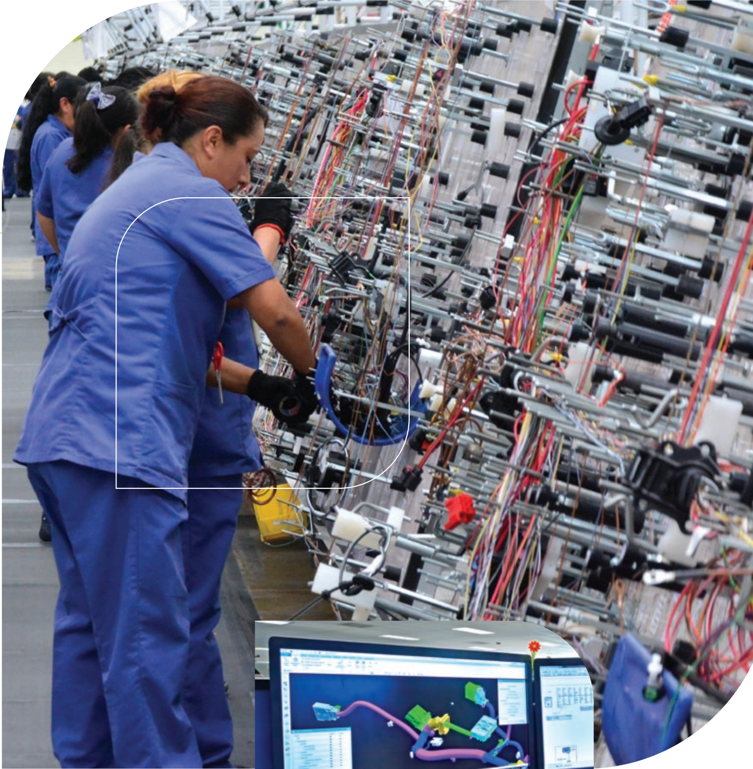
Automotive Harnesses at Arcomex Plant
